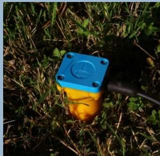
**4.5 Hz high-sensitivity vertical geophones** installed with 75mm steel spike, 1m lead-in cable, terminated with Split Spring on the end.
