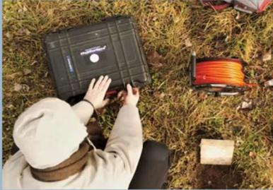
**24-channel seismograph** with a 24 bit data acquisition board and USB interface for external PC
