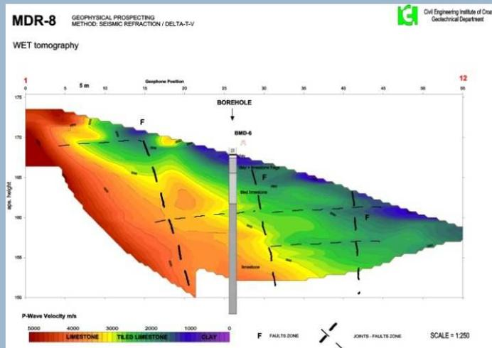
**Refraction Tomography software** that allows reliable imaging of subsurface velocity structure including faults, strong lateral velocity variation and other velocity anomalies.
