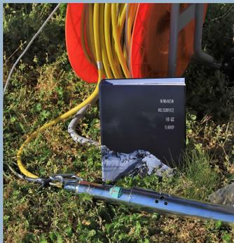
**Twin geophone** with two 3D geophones at 1m distance from each other, cable available in different lengths (50m, 100m or 150m)
