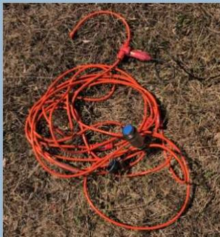
**4-ch seismic cable** ideal for MAAM acquisitions, a sort of mini-ESAC (passive seismic) and very useful and practical in many other active and passive applications.
