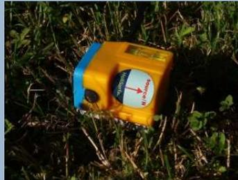
**4.5 Hz high sensitivity horizontal geophones** installed with 75mm steel spike, 1m lead-in cable, terminated with Split Spring or Mueller on the end.
