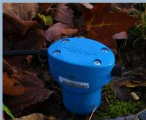
Ideal for **MAAM** (*Miniature Array Analysis of Microtremors*) acquisitions, namely a sort of mini-ESAC (passive seismic) done with 4 or 6 vertical geophones coupled with our 3-component geophone (HOLI3C) and very useful when the available space is limited
