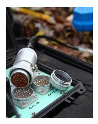
The NK-27 connector can be connected directly to the seismograph we recommend (see photo on the left) or to the final connector or the 9 channel cable we provide in particular (but not only) for the *HoliSurface®* method (see section "Holi3C for the acquisition of active data").
