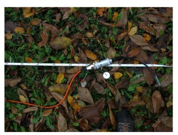
The orange cable is the *holi seismic* cable that ends with a Cannon connector that can be used to connect the **Holi3C** geophone.
