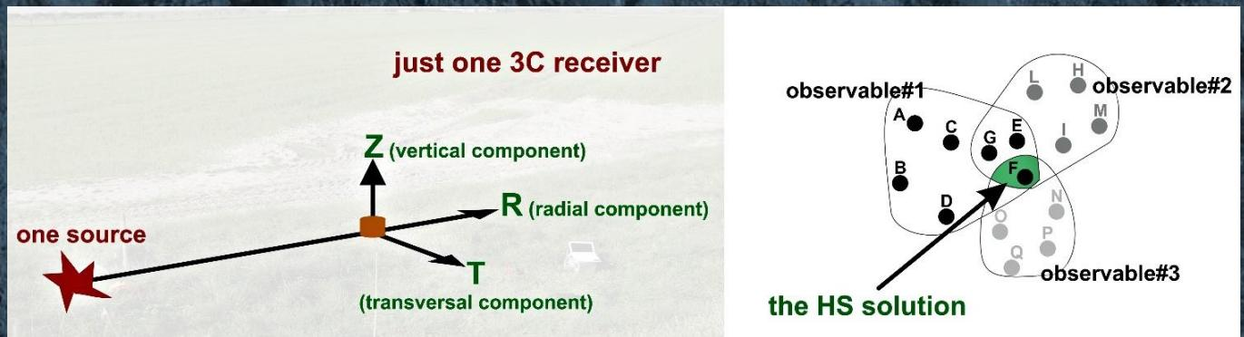
**JOINT INVERSION OF THE GROUP-VELOCITY SPECTRA (Z + R COMPONENTS) AND HVSR
