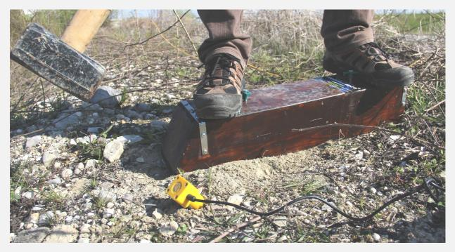
In order not to damage the wood, you can also cover the beam with the polyethylene plate used for the VF acquisitions:
