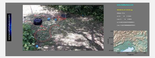
In this case, the very limited space available (see picture) required necessarily the MAAM (Miniature Array Analysis of Microtremors) + HVSR approach (which, incidentally, can be used also in case we have much more space).
