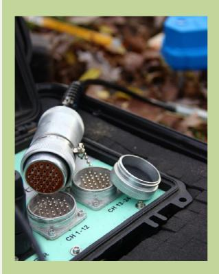
The NK-27 connector can be connected directly to the seismograph we recommend (see photo on the left) or to the final connector or the 9 channel cable we provide in particular (but not only) for the *HoliSurface*<sup>®</sup> method (see section "Holi3C for the acquisition of active data").
