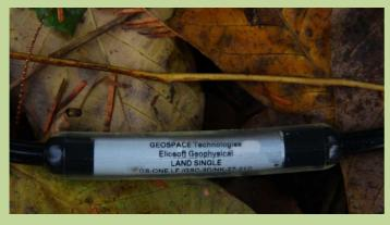
The *Holi3C* geophone is a threecomponent velocimeter designed by *Eliosoft* and realized by *Geospace* with the aim of fully meet the requirements necessary to acquire active and passive data useful for a large number of applications.
