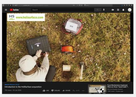
2) In case you have two 3-component geophones (see our HOLI3C geophones), you can go for the hybrid acquisition (hybrid = dataset containing both passive and active data). This way you will obtain a single 6-trace dataset to use both to extract the data for two HVSRs (at the two extreme points of the HS array), both the active data for the HS processing (see later on this manual): https://www.youtube.com/watch?v=ED gVpokZ6g
