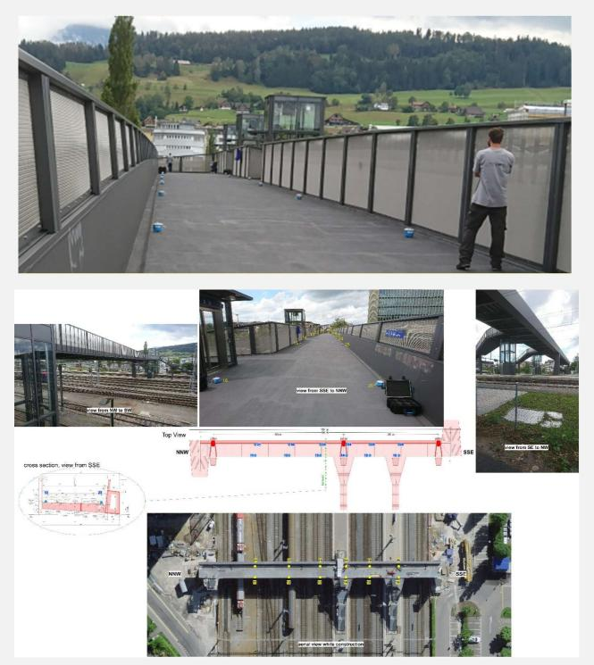
The goal is to characterize the vibration modes of the bridge (eigenfrequencies and type of particle motion).
