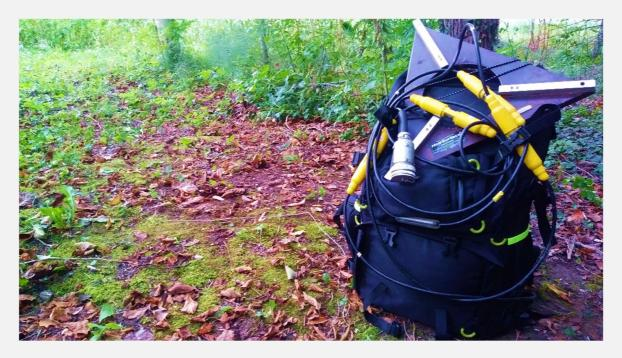
We connect the HOLI3C geophone to the end of the HoliSurface<sup>®</sup> seismic cable (see, for example, the introductory video tutorial about the HS acquisition - https://youtu.be/hqjJvAxL6xQ) and the 4 single-component geophones (in this case the vertical ones) to 4 channels of the same seismic cable, as in the scheme shown below (for the adopted nomenclature, see our Springer and Elsevier books – **dx** is the geophone spacing and **mo** the minimum offset).
