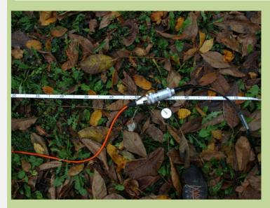
The orange cable is the 9-channel cable that ends with a Cannon connector that can be used to connect the **Holi3C** geophone.
