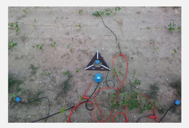
In this case our data file will have 7 traces: 3 about the 3-component geophone and 4 about the 4 vertical geophones used for the MAAM.
