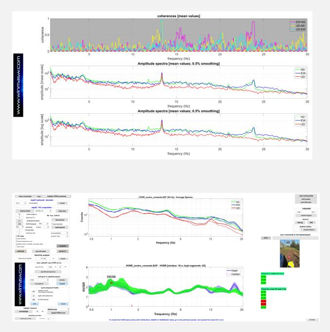
HVSR data: a couple of industrial components are apparent (they are automatically removed/attenuated - see the green curve in the bottom panel).
