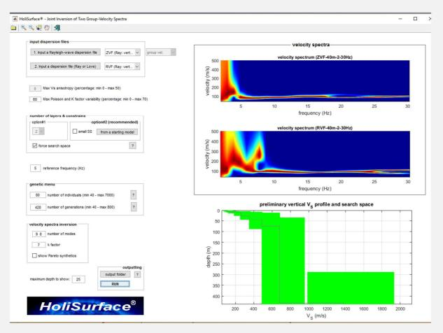
**3.** Set the number of models and generations to consider (the time needed to perform the inversion depends on these 2 values and on the power of your PC - CPU in particular - see recommendations on "system requirements")
