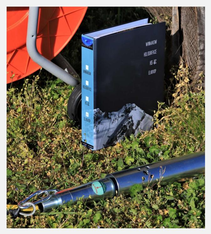
Twin borehole geophone: two 3-component geophones placed at 1 m one from the other so to halve the field effort. For details, please see the <u>ELIOVSP manual</u>, our software application for the joint analysis of downhole seismic data (P and SH arrivals) together with the HVSR.
