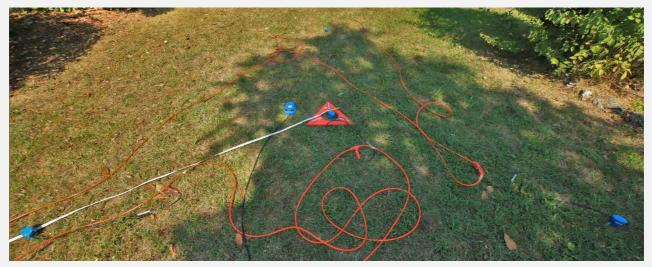
Example of a triangular array for MAAM acquisition: three geophones at the vertices of the triangle and a central one (very high-quality geophones are mandatory). Next to the central geophone you can see the 3C geophone (HOLI3C) used to determine the HVSR (which is then jointly analysed with the dispersion obtained from MAAM). All the geophones are connected to the same seismograph, thus obtaining a dataset with 7 traces efficiently managed by the *HoliSurface*<sup>®</sup> software.
