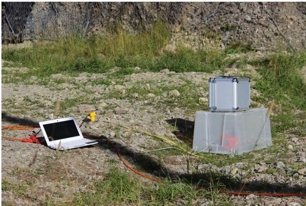
Protecting the 3C geophone against the wind
