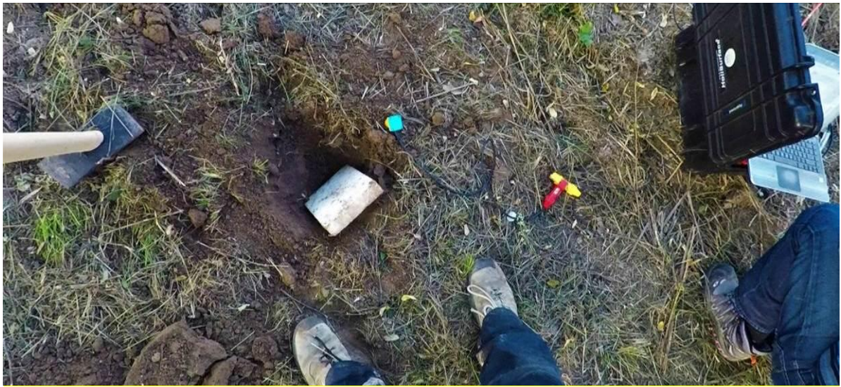
Acquisition of HF data for the analysis of Love waves and SH-wave refraction (details in the Springer book)
