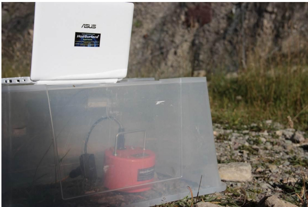
Protecting the 3C geophone against the wind
