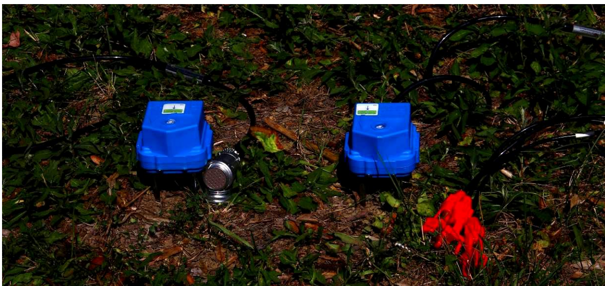
Two versions of the 3-component geophone we provide: one with a Cannon (NK27) connector (on the left), the other with three connectors (on the right).
