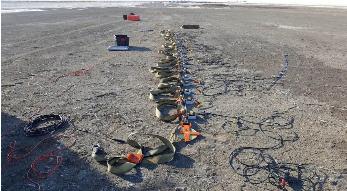
ZVF component, m_o (minimum offset): 4 m, dx (geophone distance): 0.5 m
