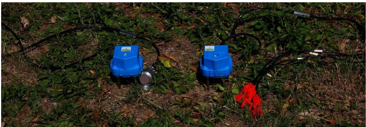
3-component HOLI3C geophone (passive geophone to connect to your seismograph)
