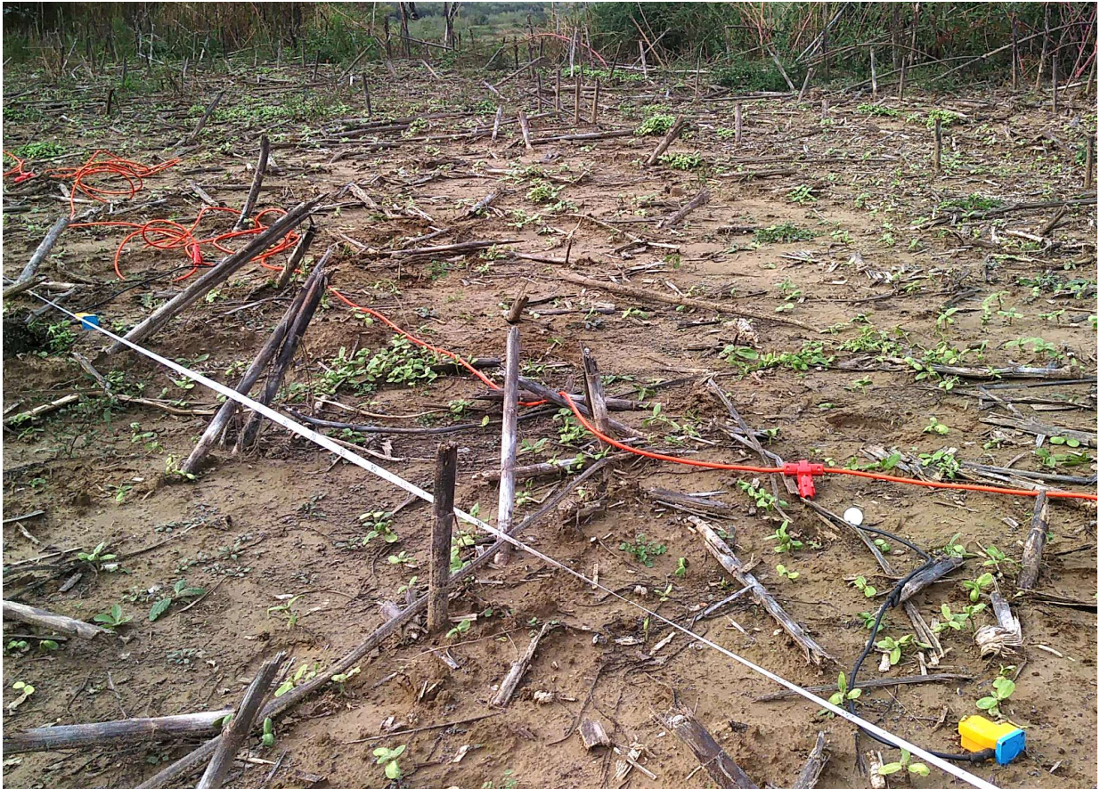
Acquisition of the R component: the axis of the horizontal geophone is parallel to the array
