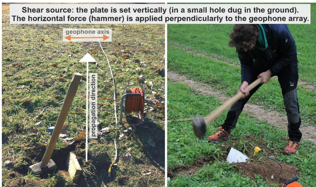
Acquisition of HF data for the analysis of Love waves and SH-wave refraction (details in the Springer book)
