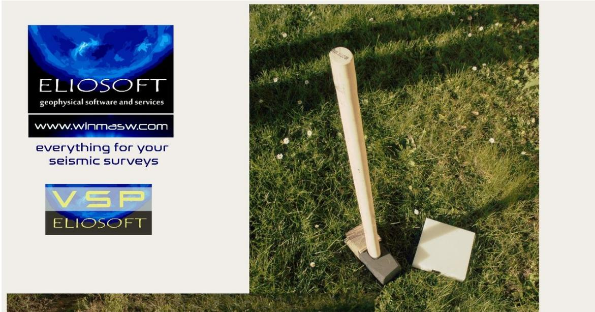
8 and 10-kg sledgehammer and polyethylene plate
